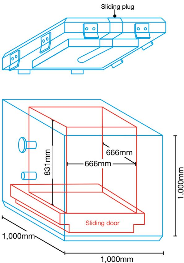
Figure 1: Dimensions of an example cuboid flask
