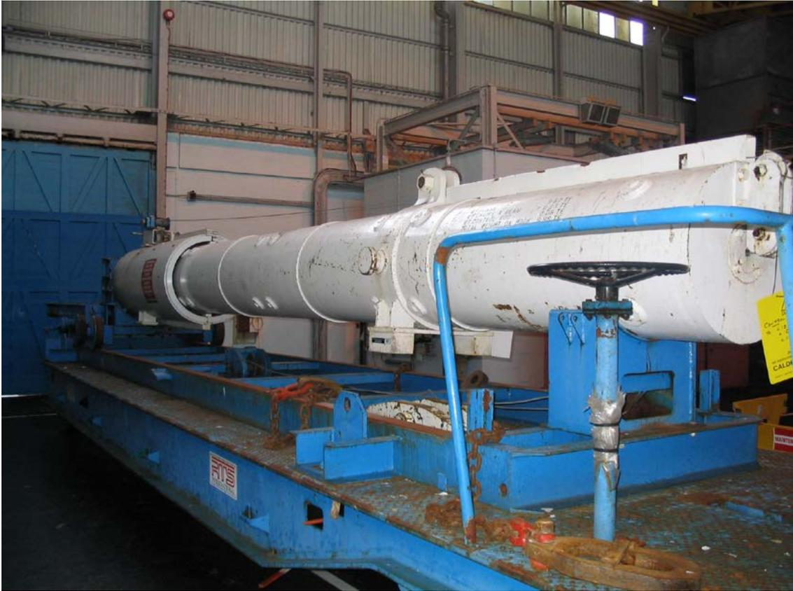
*Figure 3: Control rod flask*
