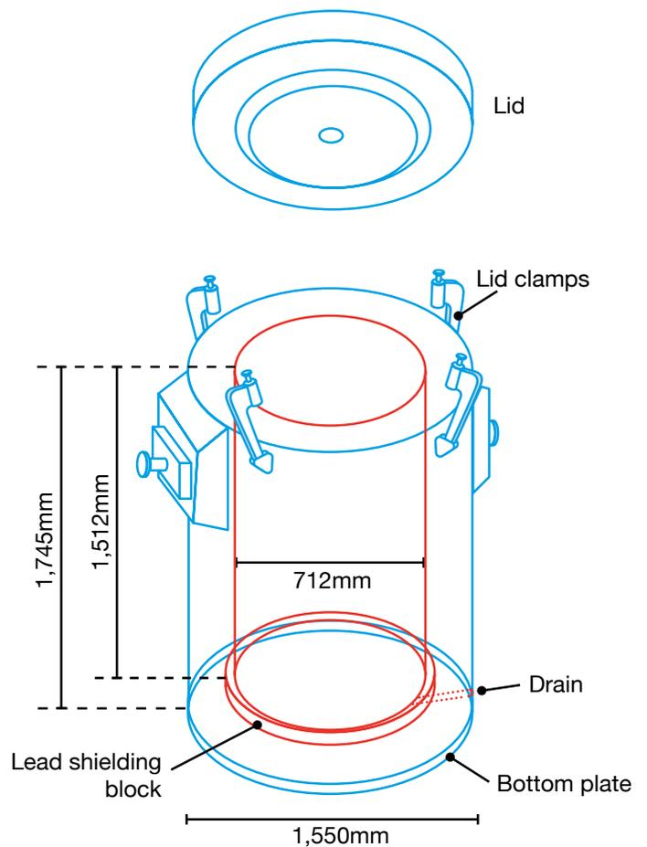
Figure 2: Dimensions of an example cylindrical flask
